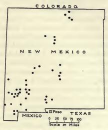
Fig. 79.—Tertiary ore deposits of New Mexico. Adapted from Lindgren and Graton: "Ore Deposits of New Mexico," Professional Paper 68, U. S. Geol. Surv., Figs. 1 and 2, p. 52 and p. 68. Note definite northeasterly belt of ore deposition.
